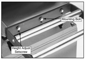
Figure 5. Extension roller attachment points.
